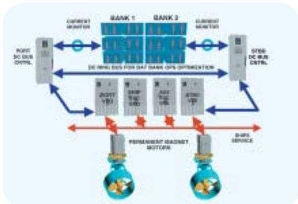
A depiction of stealth mode is shown below. The direction of the arrows indicates bi-directional current flow is possible through all areas of the distributed power. With the application of permanent magnetic motors, energy harvesting is optimized.
