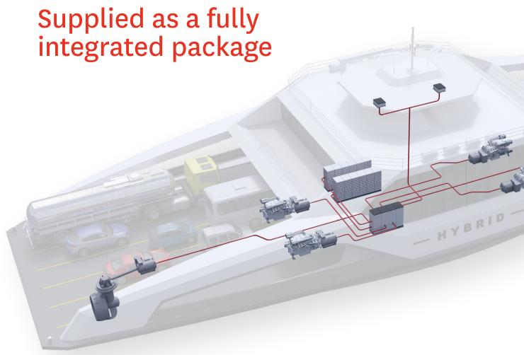
Thrustmaster supplies all the components of a marine hybrid propulsion system for the customer as a fully integrated package.
